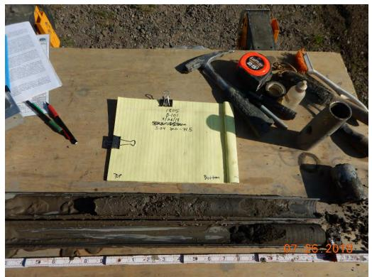
Photograph 13: B-101(P); S-24 from 70.0 to 71.5 feet. Lean Clay [Alluvium/Colluvium].
