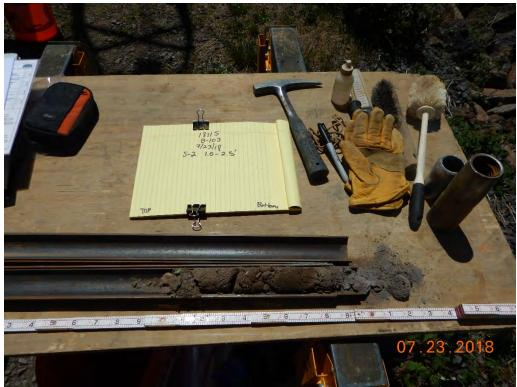
Photograph 32: B-103(P); S-2 from 1.0 to 2.5 feet. Clayey Sand with Gravel [Fill].
