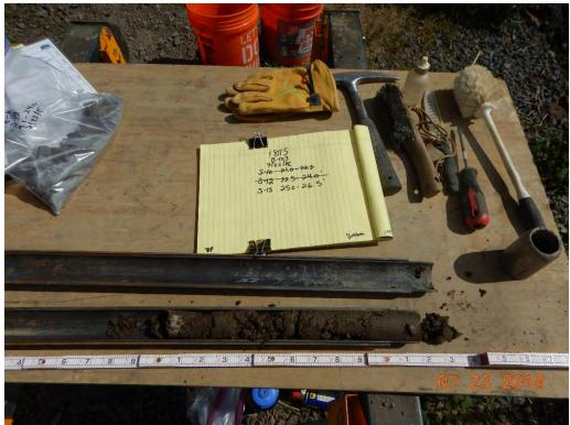
Photograph 40: B-103(P); S-13 from 25.0 to 26.5 feet. Gravelly Lean Clay with Sand [Alluvium/Colluvium].
