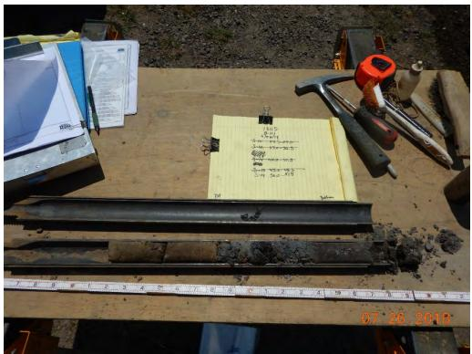
Photograph 11: B-101(P); S-19 from 50.0 to 51.5 feet. Clayey Sand with Gravel [Fill]. Sandy Lean Clay with Gravel [Alluvium/Colluvium].
