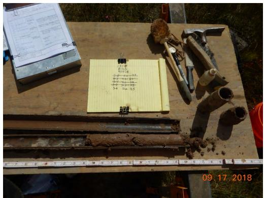
Photograph 52: B-105A(P); S-6 from 12.0 to 13.5 feet. Sandy Lean Clay with Gravel [Alluvium/Colluvium].
