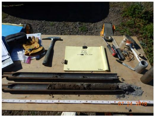
Photograph 23: B-102A(P); S-11 from 21.5 to 23.0 feet. Clayey Gravel with Sand [Fill].
