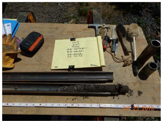
Photograph 35: B-103(P); S-5 from 7.5 to 9.0 feet. Clayey Sand with Gravel [Fill].
