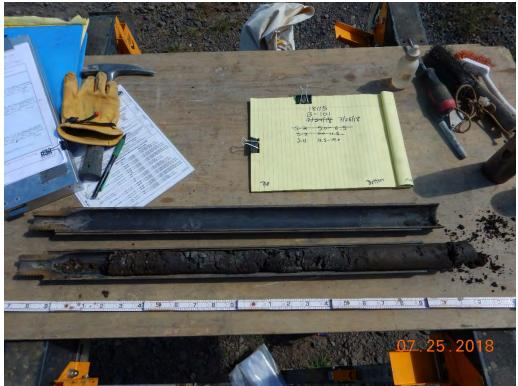
Photograph 3: B-101(P); S-3 from 12.5 to 14.0 feet. Clayey Sand with Gravel [Fill].
