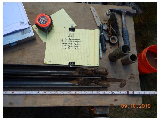
Photograph 59: B-105A(P); S-15 from 57.0 to 58.5 feet. Clayey Sand with Gravel [Alluvium/Colluvium].
