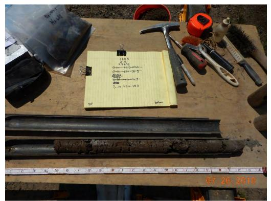
Photograph 10: B-101(P); S-18 from 45.0 to 46.5 feet. Clayey Sand with Gravel [Fill].
