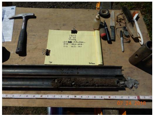
Photograph 25: B-102A(P); S-13 from 26.5 to 28.0 feet. Clayey Sand with Gravel [Fill].
