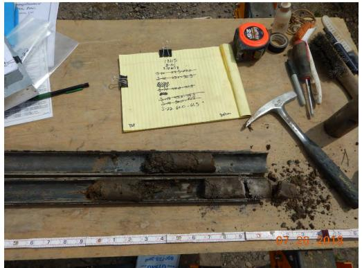
Photograph 12: B-101(P); S-22 from 60.0 to 61.5 feet. Sandy Lean Clay with Gravel and Poorly Graded Sand with Clay and Gravel [Alluvium/Colluvium].
