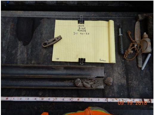
Photograph 41: B-104(P); S-1 from 4.0 to 5.5 feet. Basalt [Alluvium/Colluvium].
