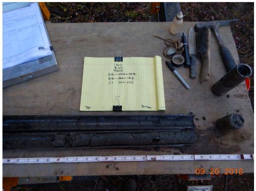
Photograph 46: B-104(P); S-7 from 22.0 to 23.5 feet. Lean Clay with Gravel [Alluvium/Colluvium].
