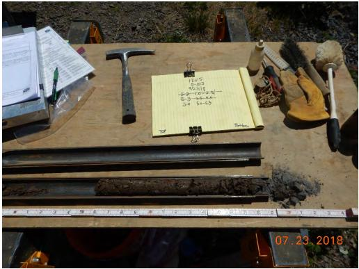
Photograph 34: B-103(P); S-4 from 5.0 to 6.5 feet. Clayey Sand with Gravel [Fill].
