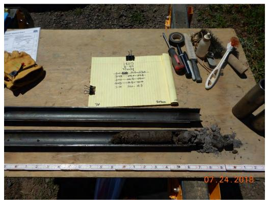
Photograph 27: B-102A(P); S-16 from 34.0 to 35.5 feet. Clayey Gravel with Sand [Fill].
