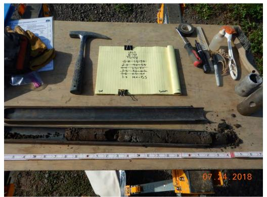
Photograph 21: B-102A(P); S-7 from 14.0 to 15.5 feet. Clayey Gravel with Sand [Fill].
