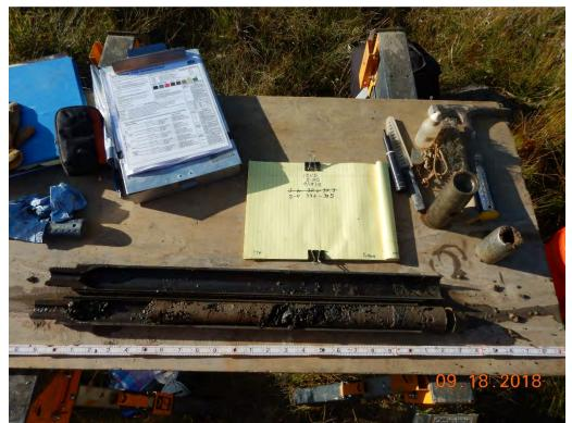
Photograph 57: B-105A(P); S-11 from 37.0 to 38.5 feet. Sandy Lean Clay with Gravel [Alluvium/Colluvium].
