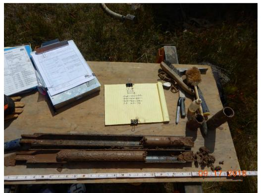
Photograph 51: B-105A(P); S-5 from 10.0 to 11.5 feet. Sandy Lean Clay with Gravel [Alluvium/Colluvium].
