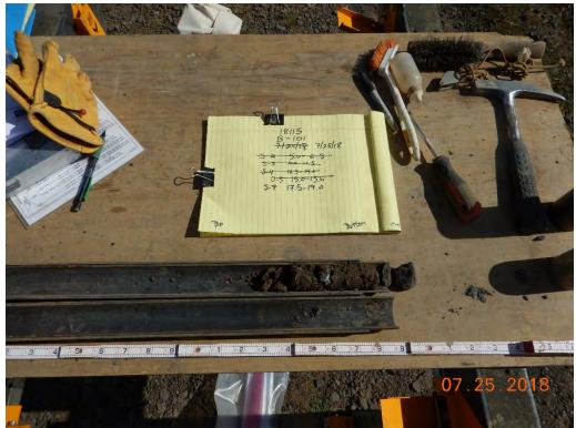
Photograph 5: B-101(P); S-7 from 17.5 to 19.0 feet. Clayey Sand with Gravel [Fill].
