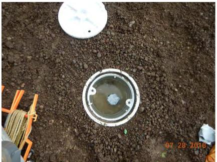
Figure 2. Duct tape covering well opening at B-101.
