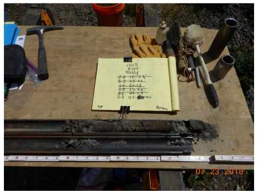
Photograph 37: B-103(P); S-7 from 12.5 to 14.0 feet. Clayey Sand with Gravel [Fill].
