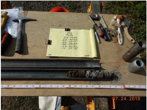
Photograph 22: B-102A(P); S-8 from 16.5 to 18.0 feet. Clayey Gravel with Sand [Fill].
