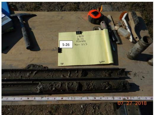
Photograph 15: B-101(P); S-26 from 76.0 to 77.5 feet. Sandy Lean Clay [Alluvium/Colluvium].
