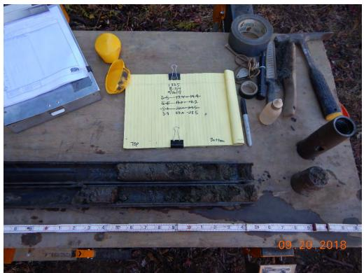
Photograph 47: B-104(P); S-8 from 27.0 to 28.5 feet. Sandy Silt with Gravel [Alluvium/Colluvium].
