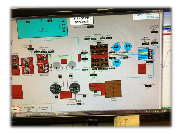
The plant is designed for an average flow of 12.5 MGD and a population of approximately 125,000. The plant was designed to be expanded to a 25 MGD plant. Other features of the plant include the use of solar panels on the Operations Building for building heating, the use of plant effluent for irrigation purposes, and odor control systems at selected areas in the plant.
