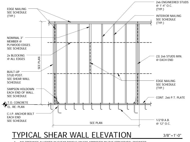
1. NO OPENINGS ALLOWED IN SHEAR PANELS UNLESS APPROVED BY THE STRUCTURAL ENGINEER. 2. ANCHOR BOLTS AT HOLDOWNS SHALL CONFORM TO ASTM F1554 GRADE 55.
