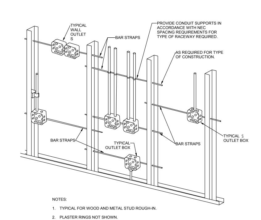
3. LOCATE ALL OUTLET BOXES IN ACCORDANCE WITH ARCHITECTURAL AND MECHANICAL DRAWINGS AND WITH ALL APPLICABLE SHOP DRAWINGS.
