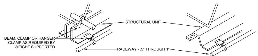
TYPICAL RACEWAY SUPPORT METHODS DETAIL
