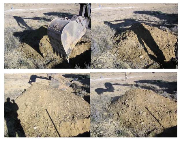
0 to 2  $\frac{1}{2}$  Feet the material was generally consistent with that of a silty sand (SM) material. 2  $\frac{1}{2}$  - 5 feet the material was a pit run cobble material (SM). 5 – 7 feet the material turned to a decomposed shale material.
