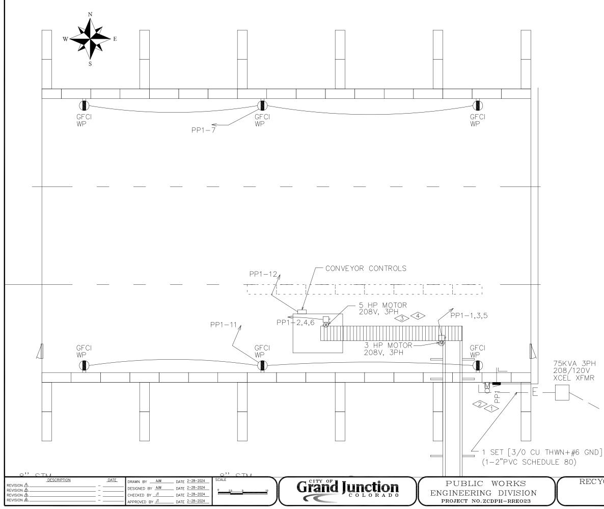
FLAG NOTES: <1> PROVIDE NEW PANEL "PP1" NEMA 3R 200 AMP 3 PH 208/120 VOLT 24 CIRCUIT NQOD OR EQUIVALENT POWER PANEL. COORDINATE INSTALLATION OF NEW METER AND PANEL WITH XCEL ENERGY. COORDINATE EXACT LOCATIONS AND WIRING, FOR CONVEYOR CONTROLS, MOTORS. COORDINATE WIRING REQUIREMENTS WITH CONVEYOR PROVIDER PRIOR TO ROUGH-IN. RECYCLING TIP FLOOR FACILITY E4 ELECTRICAL PLAN of
