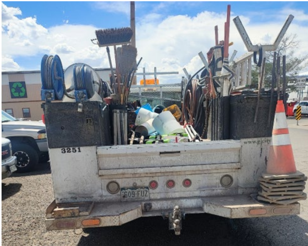
Photo of the current truck featuring the 16-inch extended rear platform-style bumper. View of the holding bracket mounted on the left side of the bumper.
